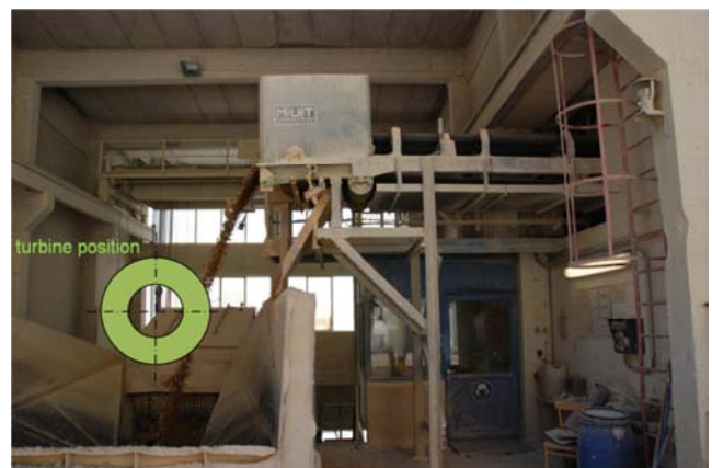
Figure 7. Transfer point from a belt conveyor to a crusher.
