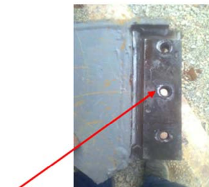
deformed threaded holes at the turbine blades
