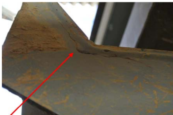
weld seam breakage at the turbine blades
