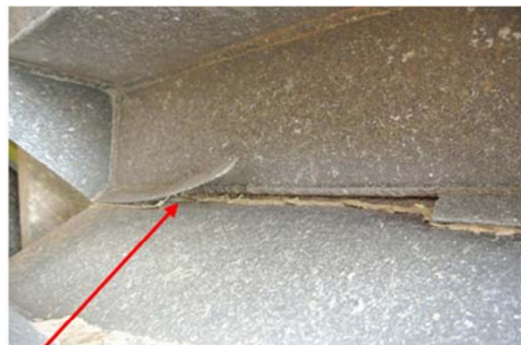
sealing slip breakage at the turbine blades
