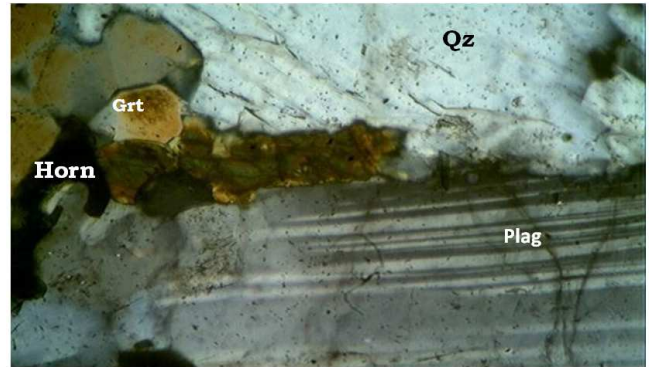
Fig.9b. Photomicrograph showing Plagioclase, quartz, garnet, hornblende XPL40
